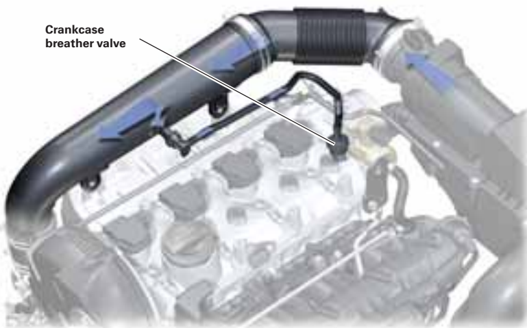
Cutaway view of crankcase breather valve
