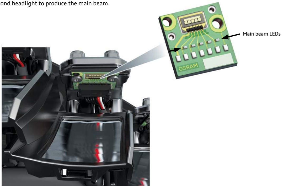
Board with main beam LEDs
