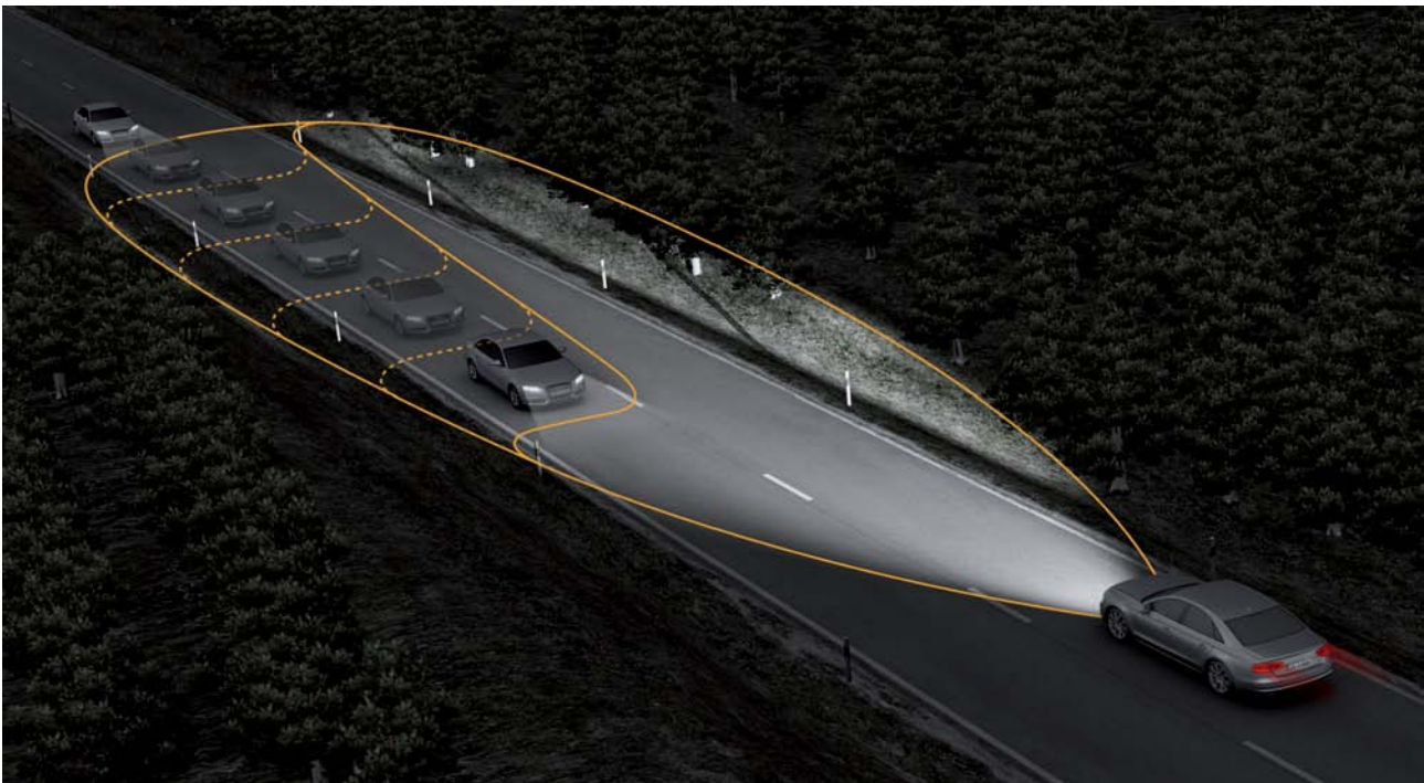
Functional principle of the intelligent light system
