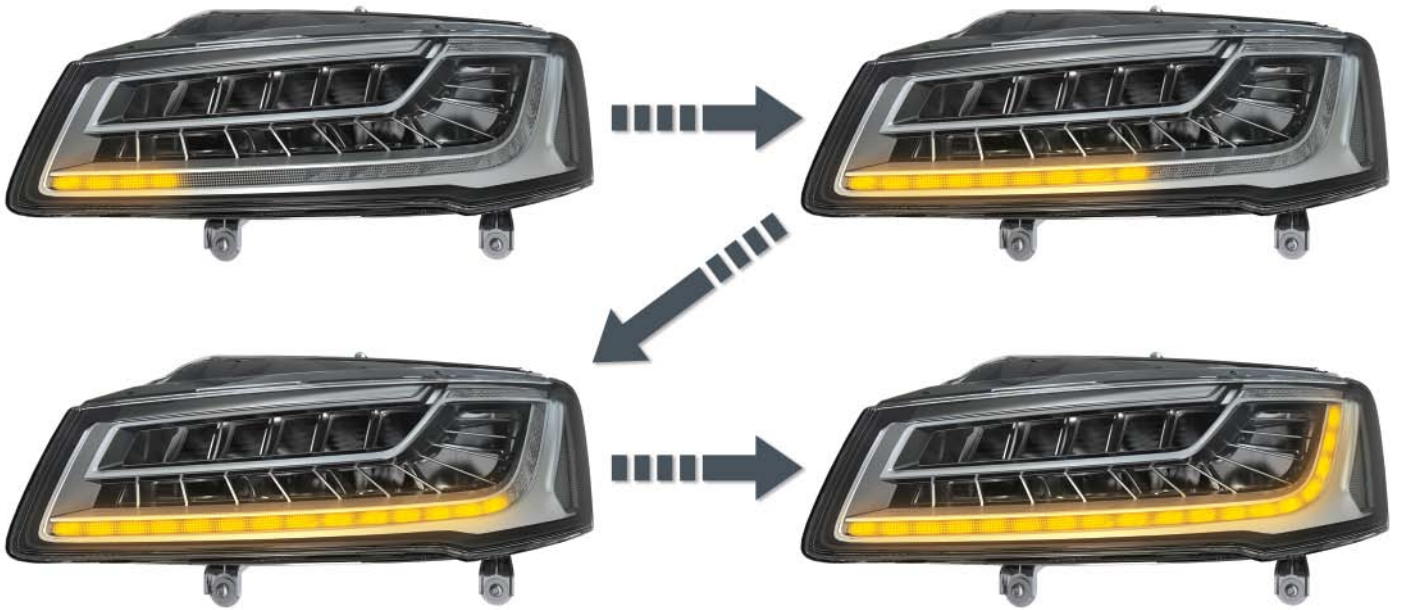
Sequential flashing with Audi Matrix LED headlights
