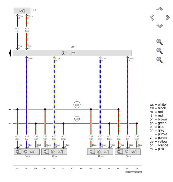
Rear centre left parking aid sender, Rear right parking aid sender, Rear parking aid warning buzzer, Parking aid control unit, Park assist steering control unit
