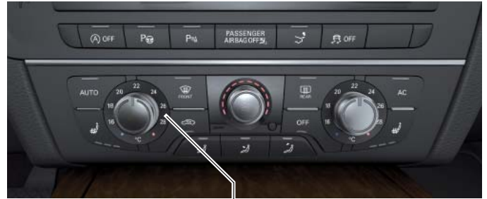
Control knob with temperature scale according to country specification
