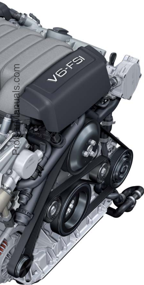
Adapted belt drive (without power steering pump)
