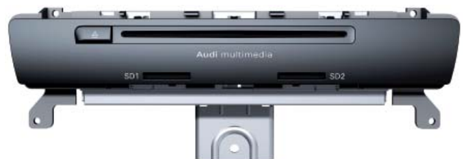
Front panel of J794 for MMI Radio plus 478_099
