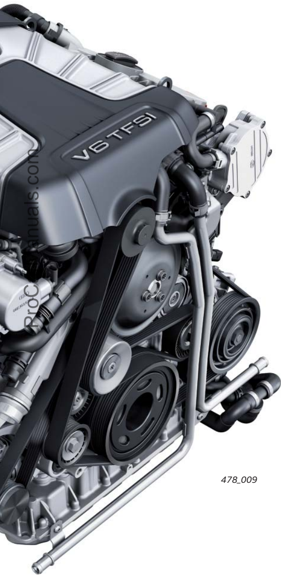
Adapted belt drive (without power steering pump)
