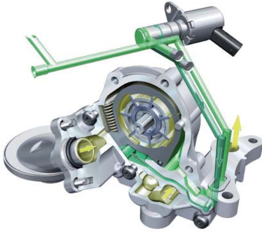
Oil pump with reduced power consumption
