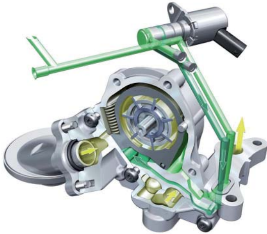
Oil pump with reduced power consumption
