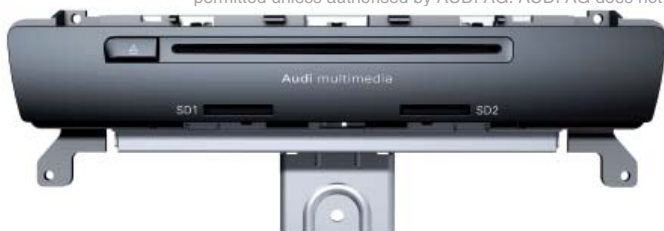
Front panel of J794 for MMI Navigation 478_099
