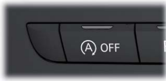
Start-stop system and brake energy recuperation
