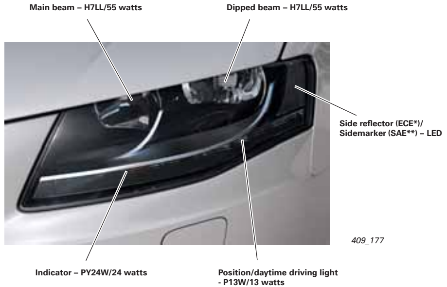
Lamp configuration in the halogen headlight version
