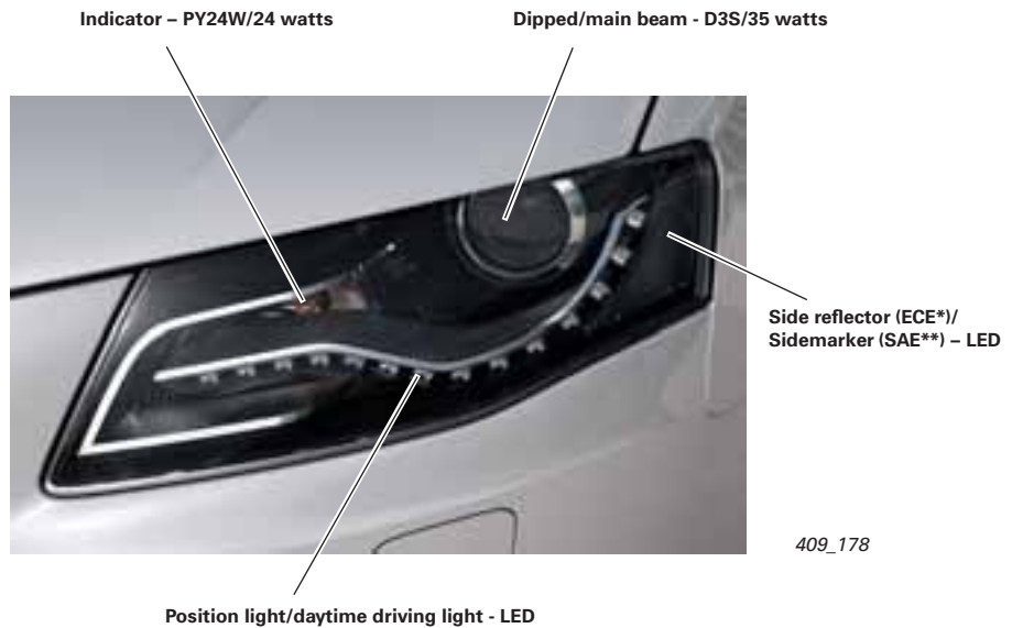
Lamp configuration in the bi-xenon version and in the bi-xenon version with adaptive light
