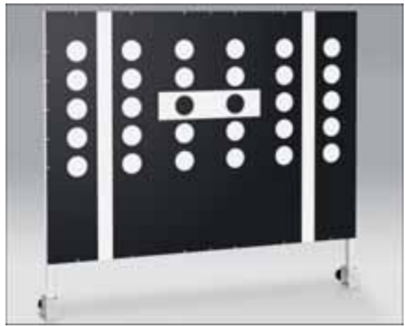
VAS 6430/4 Audi lane assist calibration board
