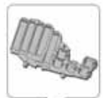
Relay and fuse panels in luggage compartment on right
