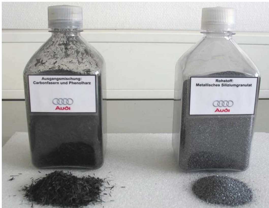
Primary materials: a compound of carbon fibers, phenolic resin and silicon granulate
