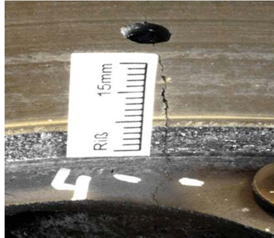
Critical interfacial crack propagation characteristic S441_028
