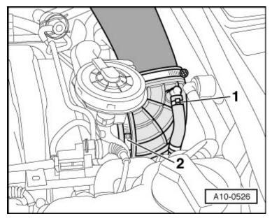
Remove hose -1- from air cleaner by turning it in direction of -arrow-. Removing Page 3 of 10
