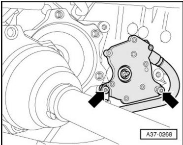
Prise selector lever cable off selector shaft lever -arrow- using removal lever -80-200-.
