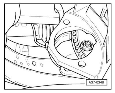
Remove multi-function switch -F125from gearbox -arrows-.
