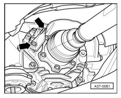
Unscrew engine speed sender -G28- (arrow B-) at front left of gearbox. Removing Page 5 of 10
