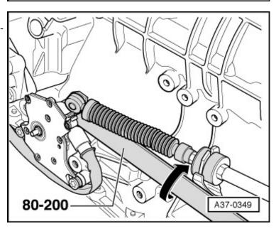
Mark position of support bracket securing selector lever cable to Removing Page 7 of 10
