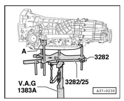
Remove gearbox support (left-side) together with gearbox mounting.
