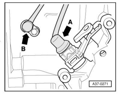
Attach electrical connector to multifunction switch -F125--item 1-. Installing Page 5 of 6
