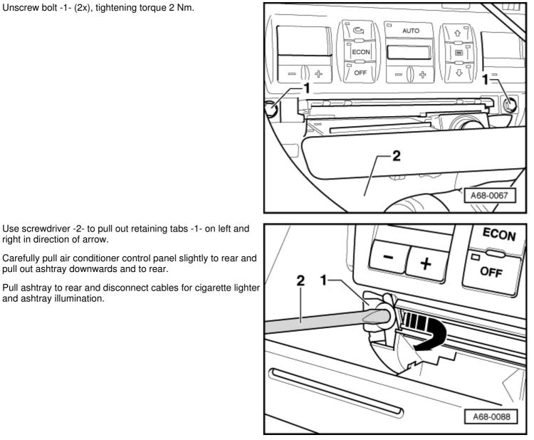
On installation, make sure guide -1- engages on left and right in centre console.
