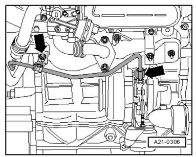
Unscrew securing nut accessible from above -1- connecting turbocharger to exhaust manifold and remove turbocharger.
