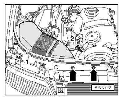
□ Unplug electrical connector -1- at air mass meter -G70-.
