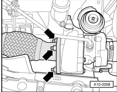
Unscrew oil supply pipe at turbocharger and exhaust manifold -arrows-.
