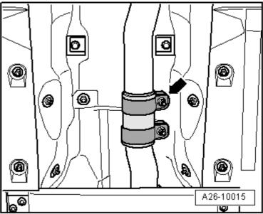
☐ Disconnect air intake hose from turbocharger -arrow-.
