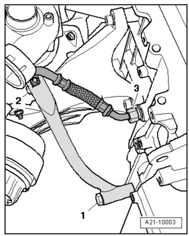
☐ Unscrew nuts -2- and -3- (accessible from below) connecting turbocharger to exhaust manifold.
