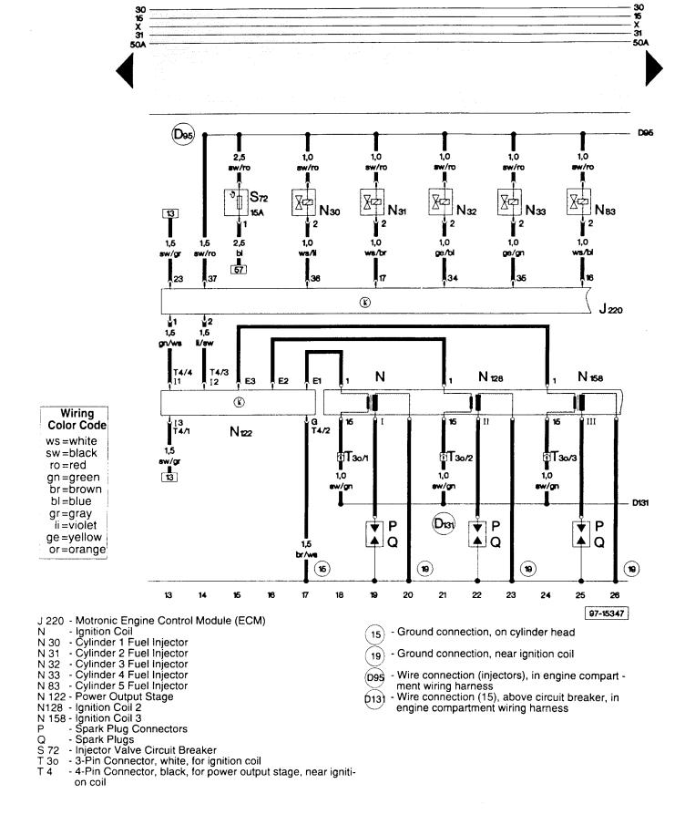
5-Cyl., ECM (Electronic Control Module) Ignition coils
