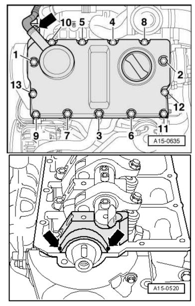
Apply one drop of sealant (Ø approx. 5 mm) to each – sealing point at front bearing cap/cylinder head -arrows-; for sealant refer to → Electronic parts catalogue.
