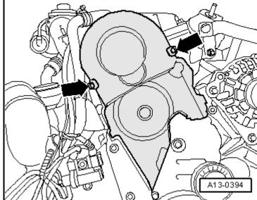
Remove top toothed belt cover by releasing retaining clips - arrows-.
