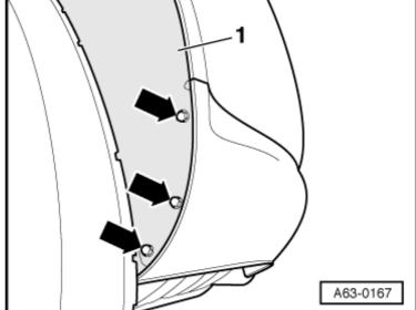
Unscrew hexagon bolts -arrows- from wheel housing liner -1-.
