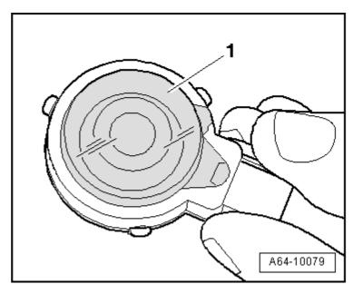
Clean contact surface of sensor on windscreen using cleaning solution D 009 401 04.
