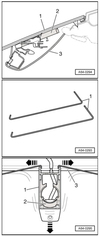
Press rain sensor with connecting cable away from windscreen to rear towards passenger compartment.
