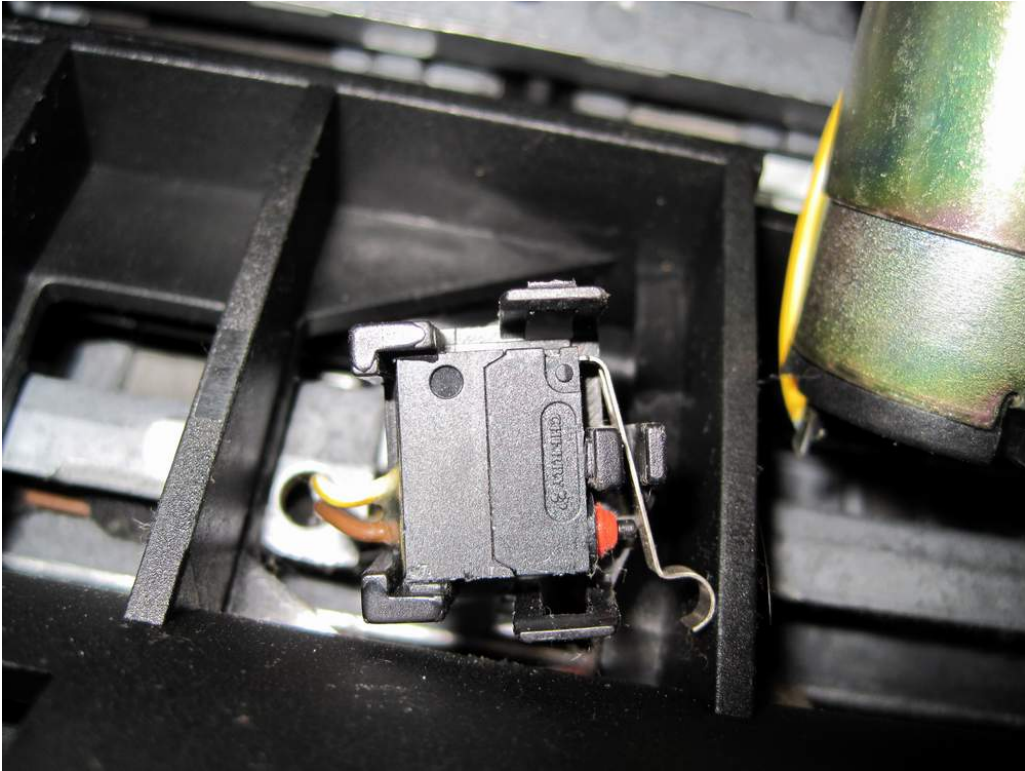
Unclip the second switch plastic housing in the same way, and remove it.
