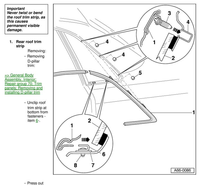
retaining clip <u>4</u>-, centre guide pin and finally upper guide pin item <u>3</u>from inside vehicle - Pull roof trim strip off guide pin of roof trim strip at front and detach. When installing, re-seal
