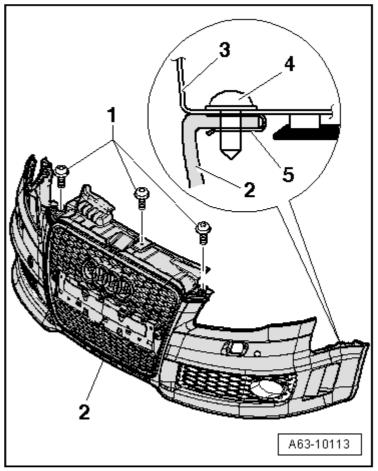
Unfasten bolts/quick-release fasteners -1and -2-. Leave rear noise insulation -quickrelease fasteners 3- in position.
