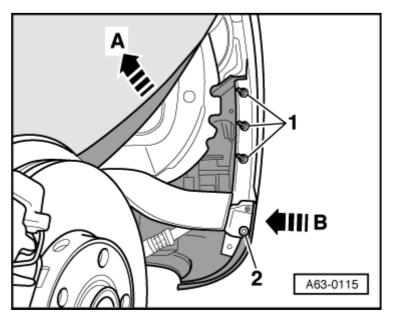
Tighten bumper retaining bolts on left and right -arrow- (23 Nm). Install air inlet grille (left and right) in bumper.
