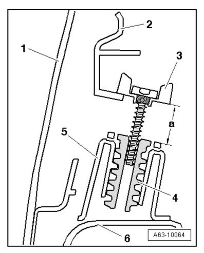
Slacken off bumper retaining bolts on left and right by approx. 15 turns -arrow-.
