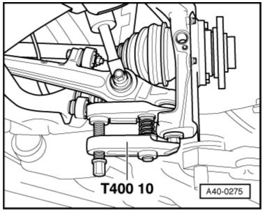
Remove nut -1-, take out hexagon bolt and pull out both upper links -2- upwards. Do not attempt to enlarge slots in wheel bearing housing using a chisel or similar.
