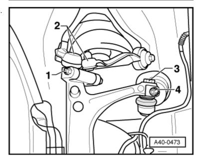
Do not apply a chisel or similar tool between steering arm -1- and seal -2- on
