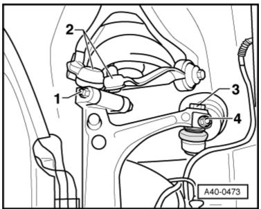
Fit splash plate and tighten bolts → Item.
