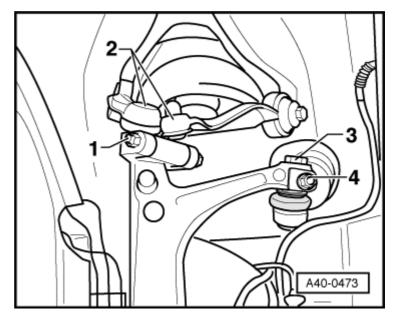
The track rod/ball joint must be inserted into the steering arm -1- by hand. Make sure that no force is applied to seal -2-.
