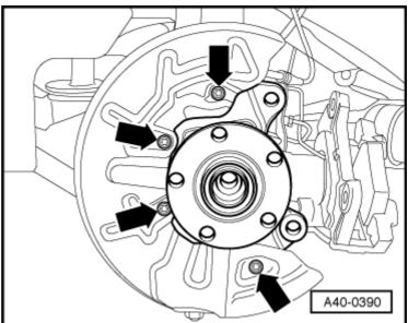
Unscrew bolt with washer -3- and bolt -4-.
