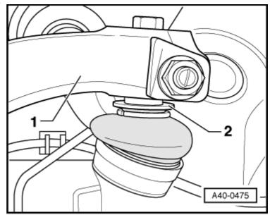
Press joint pin of guide link out of tapered seat using ball joint puller -T40010-.
