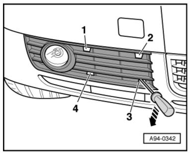
→ Release fasteners -1...4- by applying screwdriver -arrow- and pull off air inlet grille on left and right in lower section of bumper.
