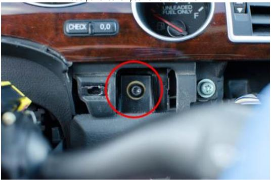
IMPORTANT STEP: There is an airbag in this lower trim panel, be careful! You don't have to completely remove the panel to access the screws.
