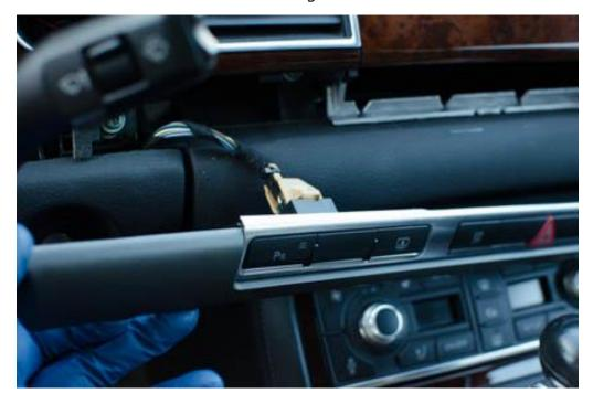
Remove the HEX Screw above the Ignition area. You can use the hex key that is on the fuse panel cover you removed earlier.
