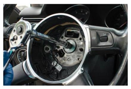
Take your fine point sharpie marker and mark the steering wheel and pinion in two spots. This will help you line up the steering wheel later.
