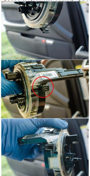
Remove the T8 Torx Screw holding the back of the unit to the others. It is located between the turn signal stalk and cruise control stalk.
