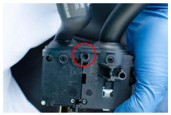
Take your T8 Torx and remove the 5 small screws attaching the units together.
