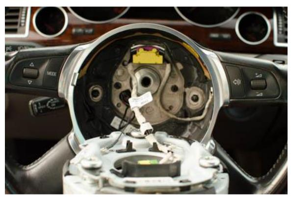
Remove the three connectors carefully as they are all different in how they connect.
