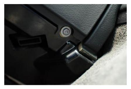
Open the change pocket drawer on the dash and remove the cover on it by gently sliding it towards the steering wheel and it will come right off.
