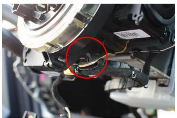
The whole unit will slide off of the column. Now we need to gently remove the three connectors from the back of the units.
