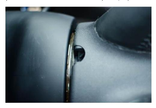
Remove the Torx Screws that hold the airbag in, the airbag won't fall out, there is an indentation on the bottom of the steering wheel column that allows easy access to the screws.
