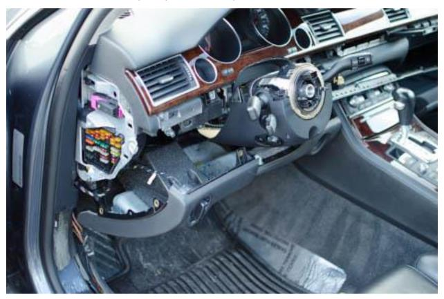
Take your T25 Torx Drive bit and remove the two screws on the bottom of the steering
