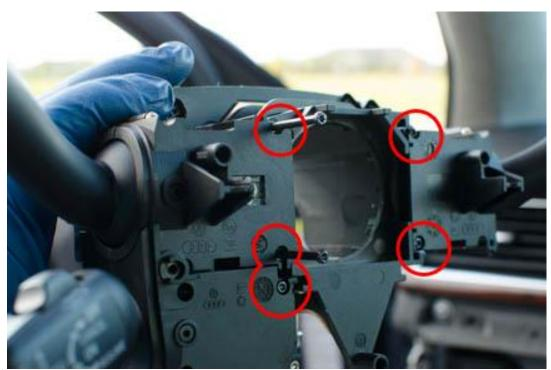
The back of the unit slides out and the three assemblies can be taken apart.
