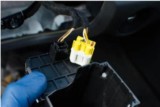
GENLTY pry the three clips that attach the clockspring to the unit.
