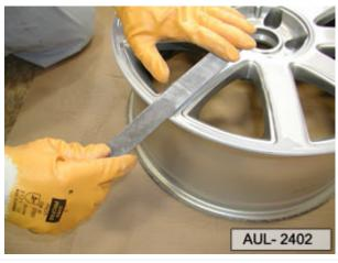
Use a file or orbital sander to roughen the damaged area. This ensures complete removal of the existing paint and produces the required 120 grit size peak-to-valley height. Deep scratches and notches must always be filed down and rounded off to avoid a notching effect. The area immediately surrounding the repair location should also be thoroughly surface-sanded to ensure adhesion of the feathered-out filler material.
