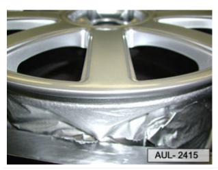
be found under <a href="https://www.vwcolor.info">www.vwcolor.info</a>. Use a metal colour sample to check the shade. Then apply water-borne base coat paint to the rim in 1-2 spray applications
