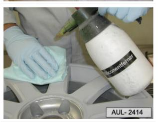
Clean the rim with silicone remover before applying the base coat paint.
