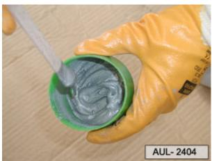
Mix a sufficient quantity of twopack Diamant aluminium filler.
