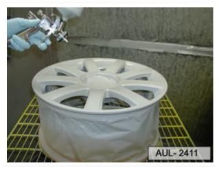
Depending on the extent of the damage, apply surfacer to the repair location or the entire rim. Only two-pack Vario surfacer is permissible for this purpose
