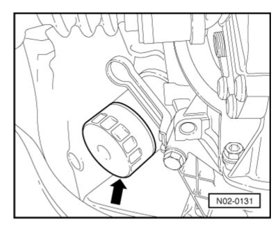
Screw in new filter and tighten.
