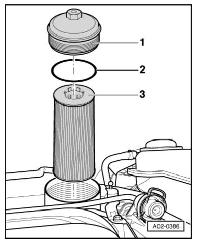
Tighten sealing cap -arrow-.
