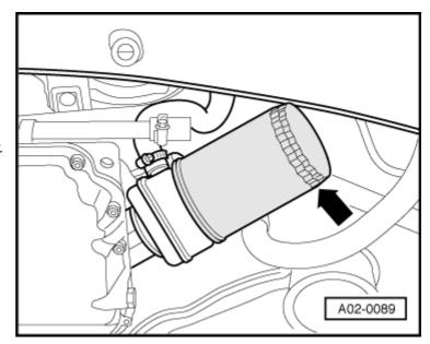
Screw in new filter and tighten.
