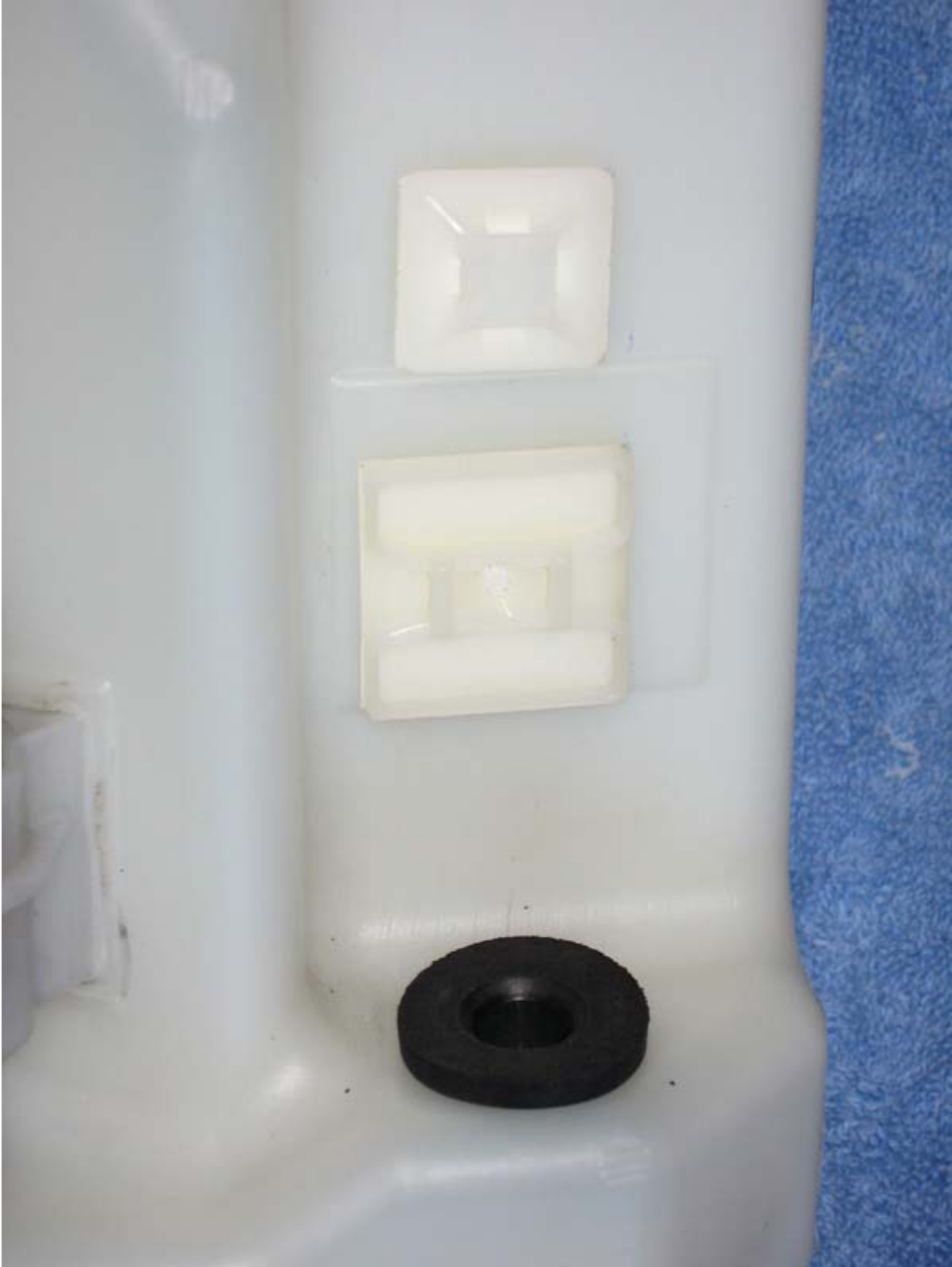
Grommet fitted to new hole, I used self adhesive "cable tie bases" to secure the pump to the washer bottle.....
