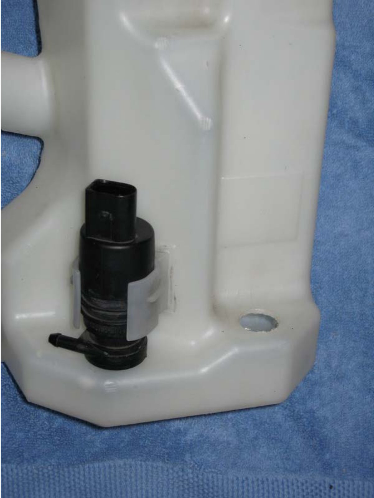
Hole drilled with a 20mm Hole cutter.....
